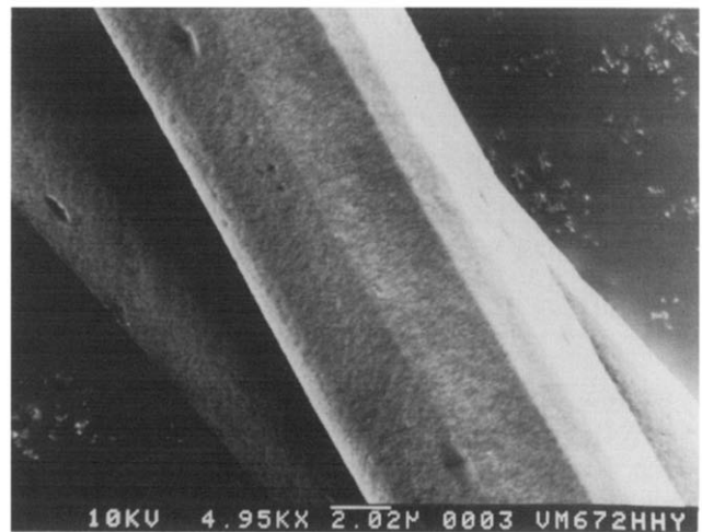
Figure 4 Scanning electron micrograph of VM after 672 h hydrolysis
